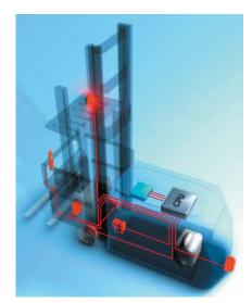
A laser scanner is installed both in direction drive and in direction lift. By means of these, the vehicle is monitored parallel to the floor at a height of ca. 20-30 cm. The laser scanners are are connected with the control electronics GM-107cpu which controls the Personnel Protection System and takes over communication with the vehicle electronics.
