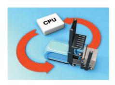
Mobile Personnel Protection System GM-107cpu consists of two laser scanners (Type Sick S 3000), a central micro-processor controlled electronic system, fitting consoles, connection and control leads, together with all necessary signal transmitters.
