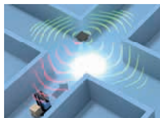
Vehicle alone: continuous light will be triggered
