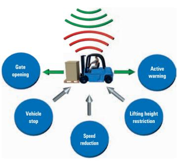
The NoColl Dome/v2 controls the vehicle functions from the driver's overhead guard. It indicates the status of the vehicle influencing by an illuminated ring that is visible from far. The integrated electronics are microprocessor controlled for redundant signal processing.
