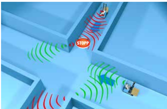
Speed reduction at intersections Safe and collision-free traffic control
